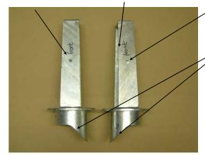
The front turrets are to be fitted with the hole and the writing facing forwards towards the bumper.
