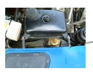
On certain models the water header tank may need spacing out to stop the top of the shock fouling the bottom of the tank.
