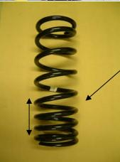
If a progressive spring is being used on the rear ensure that the coils closest together are at the bottom as this leaves more room for the hook of the re-locator to catch the spring.
