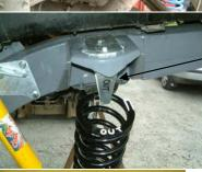
When mounting the spring ensure that the re-locator hook catches the last full coil of the spring.
