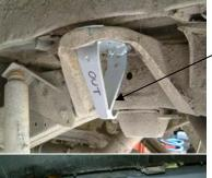
Lift the re-locator into place with the hook of the re-locator facing inwards.
