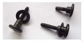
You will require the two longer shoulder bolts that are part of the seat frames on the Discovery, if you haven't got them you can make them out of an M6x35 bolt, two M6 nuts and one washer.
