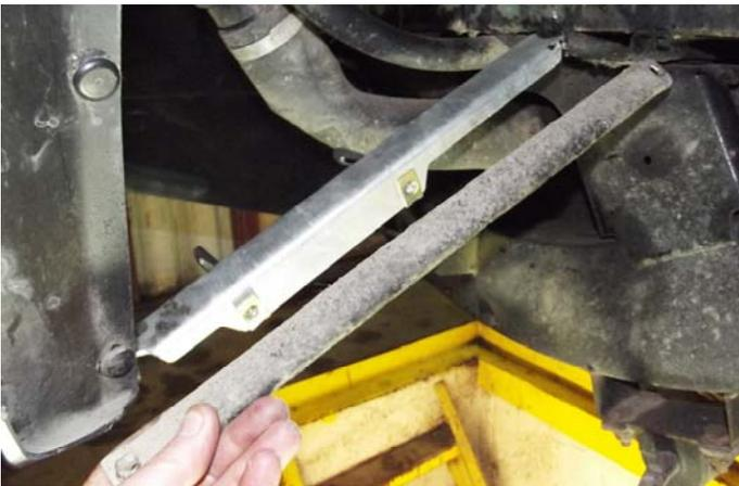
You may need to remove the original body stay before you can drill the two holes for the top mount (do not fit the new body stay as yet)
