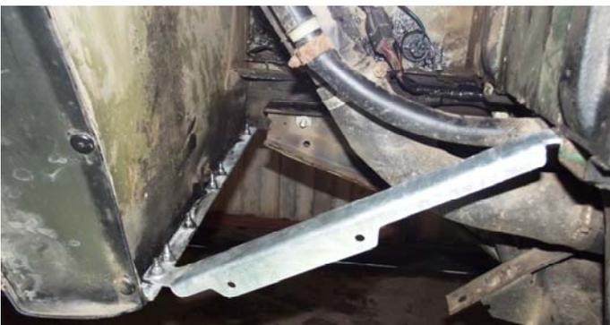
The body stay may now be fitted using M6x25mm bolts, nuts and two washers per bolt.
