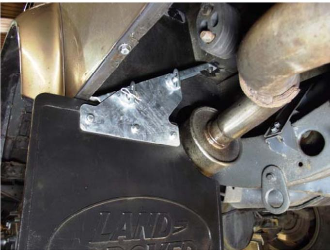
Mud flap shown fitted and cut around exhaust silencer.
