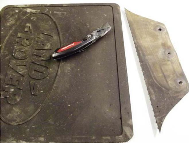
The top must be cut off both mud flaps as shown.
