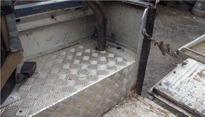
**Square Rear Tub** is all 110s from the beginning and up to 2007, Puma Td4s 2007 on mainly all commercial style ones, like crew cab pickups single cab pickups and 3 door hard top van style all have square rear tubs.
