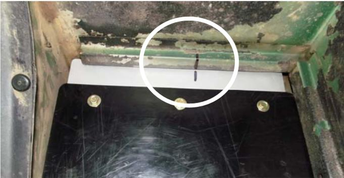
**GL1008** Temporarily fasten the mud shield to the top mounting bracket with the three speed screws as shown. Centralise the shield in the tub, make sure you are happy with the position of the shield before you drill the holes. Once you are happy with the position mark a line on the bracket and the tub as circled and remove the mud shield.
