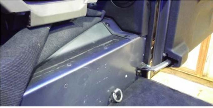
**Stepped Rear Tub** is 2007 on Puma Td4 that have seats in the very back or a 110 utility that has no bulkhead behind the 2nd row of seats, the step was put in by Land Rover for rear forward facing seats.
