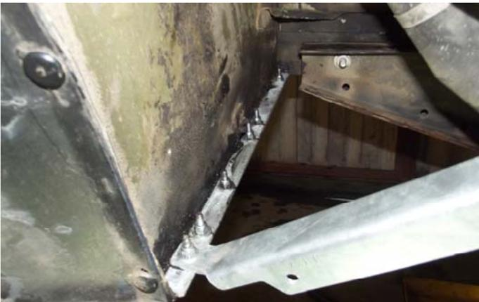
Extra holes have been drilled in this one as the lower edge had corroded. we have supplied an extra three per side incase you need them. Before you bolt the steel plate in place smear plenty of grease between the two surfaces to help stop any more corrosion.
