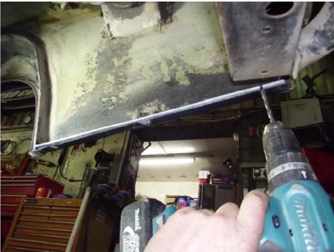
Two holes will align but you may need to drill the third hole as shown. You may find the lower edge has corroded where the original holes were, you will have to drill extra holes to secure the side panel strengthener, you would normally use just three bolts each side but extra have been supplied if you need to use them. Bolts used, M6x25mm / nylock nuts / two washers per bolt.
