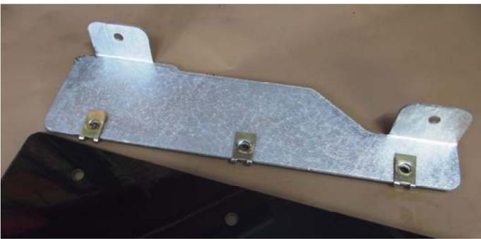
**GL1003** 110 CSW TDCI 2007 onwards with stepped tub. Fit the 3 U-Clips fasteners as shown.
