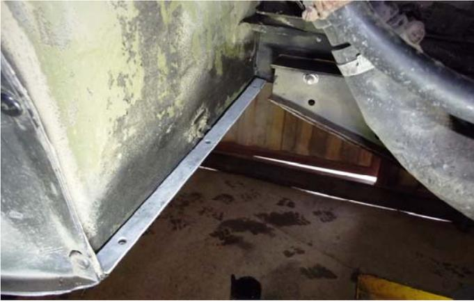
The side panel strengthener needs to be fitted next, make sure it is clean where the steel plate is to be fitted.
