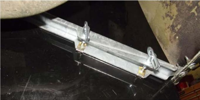
Fit two U-clips to the body stay and now the mud shield can be fully fitted in place with five speed screws. Now fit two ant-lose pins for the removable mud flap bracket.
