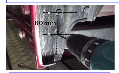
Mark out and drill a 6.5mm hole 60mm lower than the hole above as in the picture. Once this is done the rest of the fitting is done the same way
