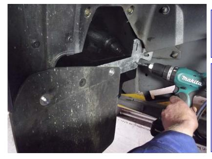
If you are using your original Front Mud Flaps you will need to remove the original metal mounting brackets, this is done by drilling out the original three rivets.
