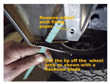
Cut the wheel arch flare as shown and remove the plastic rivet, the M6 bolt can now be fitted pointing out as in picture 2 (To remove the plastic rivet just push the pin in its centre through and catch it from round the back of the rivet)
