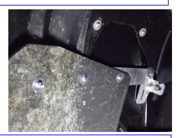
You will also mount the horizontal bracket on the upper slot of the chassis bracket
