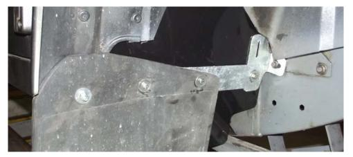
Drill the two remaining holes in the plastic shield then fit and tighten the bolts.
