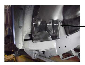
The easiest way to cut this inner arch is to follow the dashed line as in the picture to the left. Make sure you cut below the two screw fixings
