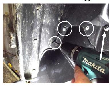
Once the shield is secured in place drill a hole in to it using a 3.5mm drill bit and replace the rivet you removed earlier with one of the supplied speed screws.
