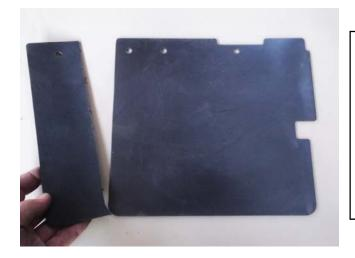
If fitting this kit to a TD5 or Puma TD4 you'll need to cut the Mud Shield to fit around the Fuel Filter. The Mud Shield has a cut line marked on the rear, use a hacksaw blade to cut this off.
