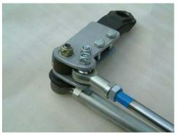
At this point the hydro assist ram can be fitted, please note the way the bolts are fitted through the bracket, if they are fitted the other way they could foul the drag link.
