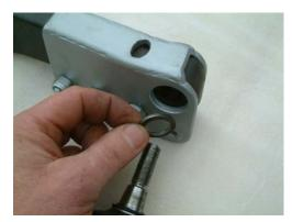
Place the new bracket over your drop arm, some grinding may be required on your drop arm as it is cast and they do vary in size, insert bolts but do not tighten at this point. Insert spacer washer over the track rod end before inserting the track rod end through the drop arm this is here to centralise the track rod end in the bracket.
