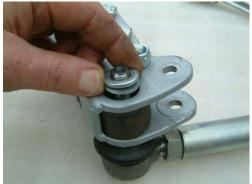
Once the track rod end is in place insert two 12 mm washers to centralise the track rod end in the top of the bracket.
