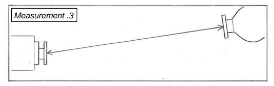
This Measurement is axle fully up to bump stops.
