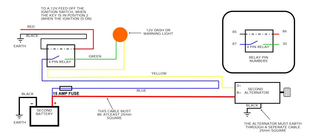
You must fit a separate earth cable from the alternator body to the engine block. This is very important to get maximum charge out of your alternator.
