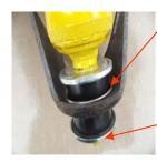
New shock isolation bush washer fitted, only ONE on each end required.
