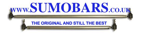
When fitting a sumo 740 extreme bar to a defender you must cut 20mm/2cm off the original steering arm as it will not screw far enough into the new sumo bar.
