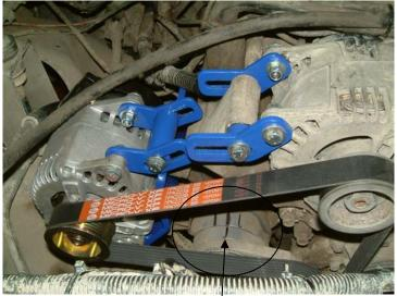
Air con tensioner (ERR3440) must be used. Both alternators can be adjusted to make sure the belt tensioner is at the centre of its travel. You must fit a separate EARTH CABLE from the alternator body to the engine block. This is very important to get maximum charge out of your alternator.
