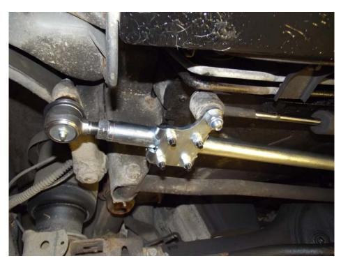
As fitted to Range Rover P38 The bracket will mount horizontally.
