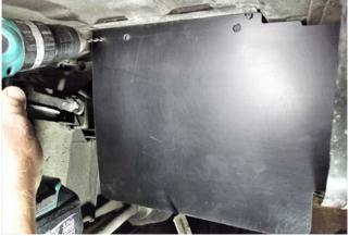
Before starting to fit these shields make sure there is no mud on the outer side panel nearest the wheel arch, this will stop the shields fitting correctly.
