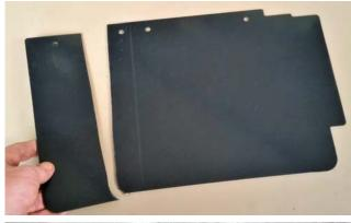
If fitting this kit to a TD5 or Puma TD4 you'll need to cut the Mud Shield to fit around the Fuel Filter. The Mud Shield has a cut line marked on the rear, use a hacksaw blade to cut this off.
