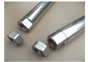
Groove on the right hand bar and nut.
