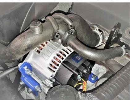
You may need to slacken this hose clip to raise or adjust the water hose so that it sits better over the alternator. (make sure the water hose remains fully secured on)
