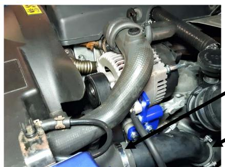
If this pipe for the intercooler touches the mount you can loosen these two hose clips and turn the pipe to give you the clearance you need.
