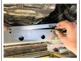
Lastly, you will be supplied with two lids to fit on top of the track rod guard. Fit all U nuts to the both lids and fit the lids to the track rod guard with the speed screws as shown on picture.
