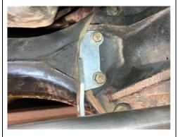
Loosely fit the front support bracket to the diff.
