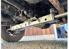
Fit track rod guard as shown in picture.
