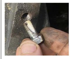
You may need to clean out the threads in your diff. To do this we have supplied one extra bolt in the kit. You can grind or file a slot in the bolt, this will act like a tap to clean out the threads.
