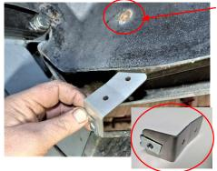
Remove the two inner wings self tapping screws on your Defender. Fit the U nut to bracket **B,** as shown on picture.
