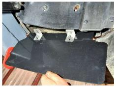
Slide the shields up between the inner wing and front wing, align bracket **A** with the hole and fit the speed screw and 25mm washer
